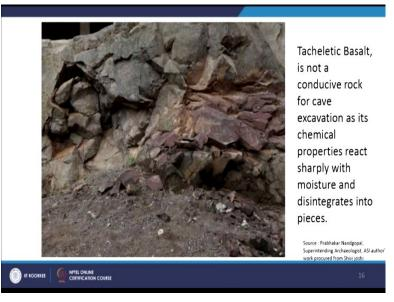
And this Tacheletic Basalt which is not a conducive rock for cave excavation as its chemical properties react sharply with moisture and disintegrate into pieces. The moment you are making an excavation process, it gradually brokes into small wedge-shaped pieces you know, that is one of the important aspect in the excavation challenges and excavation challenge especially with this kind of material.
